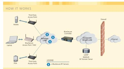
The BlueSecure Controller acts as a firewall between the wireless LAN access points and the wired LAN, and requires no changes to existing wired LAN hardware or user client software. Additional BlueSecure Controllers can be connected to provide hot failover capability, as well as scalability and subnet mobility across the enterprise.
